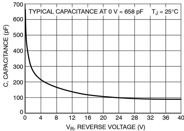
**Figure 7. Typical Capacitance**
