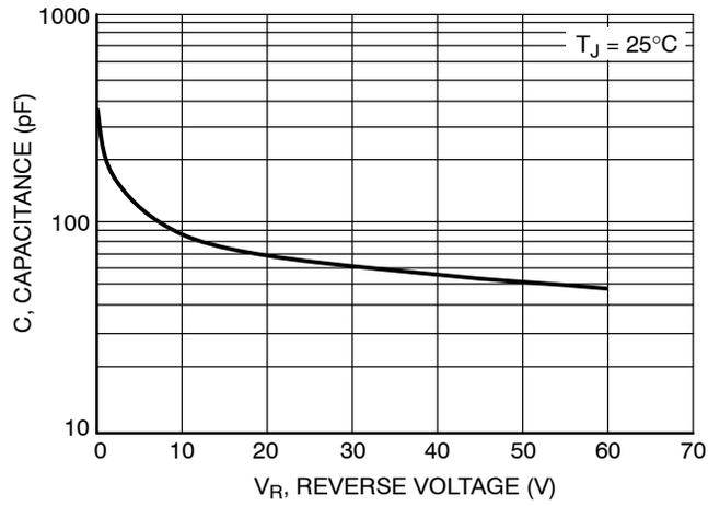
**Figure 7. Typical Capacitance**
