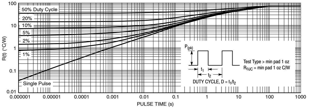
Figure 9. Typical Thermal Response, Junction-to-Ambient, SMB Package
